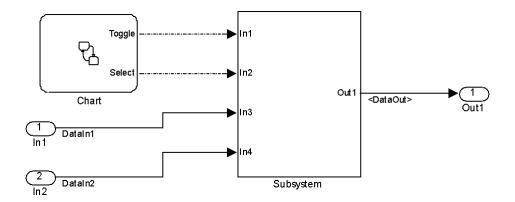
The next figure shows the contents of Subsystem in the previous figure. The subsystem contains two function-call subsystems, each driven by one of the signals input from the top level.
