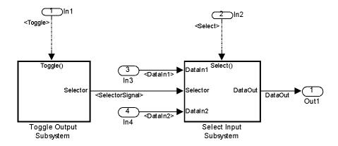
In the preceding model, the Stateflow chart can assert either of two scalar signals, Toggle and Select.
